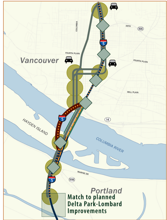
Supplemental Bridge for I-5; Bus Rapid Transit on Existing Bridge
